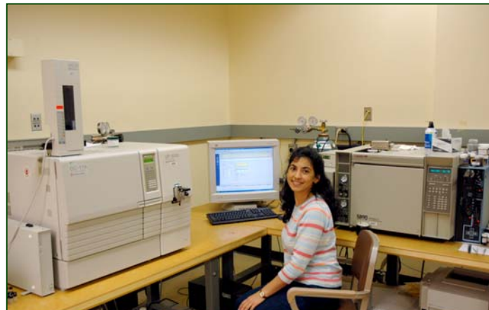
Shimadzu QP-5000 Gas Chromatography/ Mass Spectrometry featuring Direct Insertion Probe
