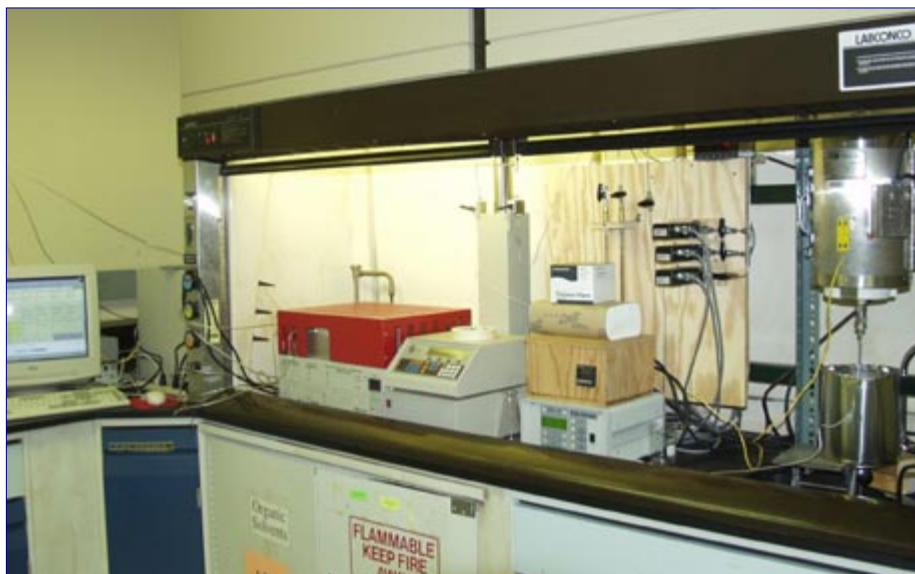
SARS System for Adsorption Desulfurization
