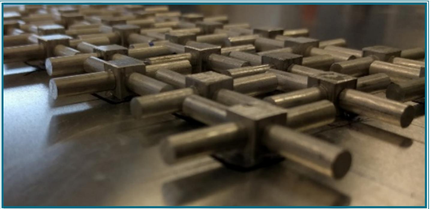
An array of resonators glued on an aluminum plate. IMAGE- Chris Hakoda
