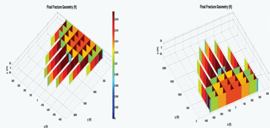
An example of hydraulic fracture network and width at the end of a stimulation treatment from Wang's hydraulic fracturing model. Image contributed by John Yilin Wang.
