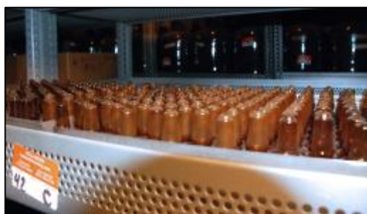
Coal samples sealed in borosilicate ampules sitting on storage shelves at the EMS Energy Institute.
