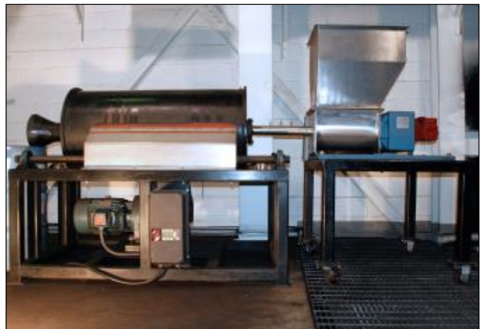
2'x4' continuous ball mill (125 lb/h)
