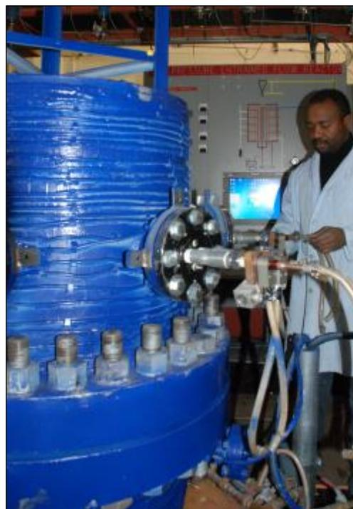
High Pressure, High Temperature Flow Reactor
