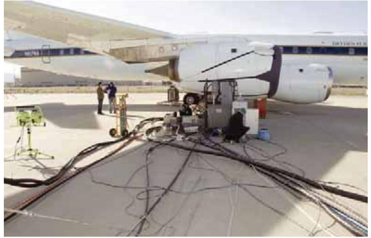
Test instrumentation was set up behind the inboard engines of NASA's DC-8 airborne science laboratory during alternative fuels emissions and performance testing at NASA's Dryden Aircraft Operations Facility in Palmdale, CA.
