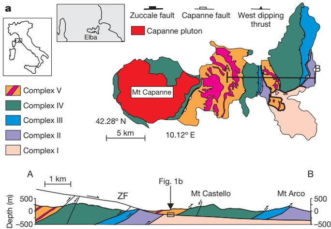
**Figure 1 | Example of a foliated low-angle normal fault.** **a**, Map and cross-section of the Zuccale fault (ZF) as exposed on the Isle of Elba, Central Italy. The Zuccale fault is an exhumed, ancient low-angle normal fault belonging to the Apenninic system. In the tectonically active area of the Apennines, to the east, a similar low-angle normal fault is producing microseismicity at
