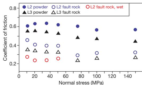
**Figure 3 | Frictional properties of fault rocks and powders made from them.** Steady-state friction plotted as a function of normal stress. The solid samples show friction values that are consistently 0.2–0.3 weaker than powders. Further weakening for intact fault rocks is achieved under water-saturated conditions.
