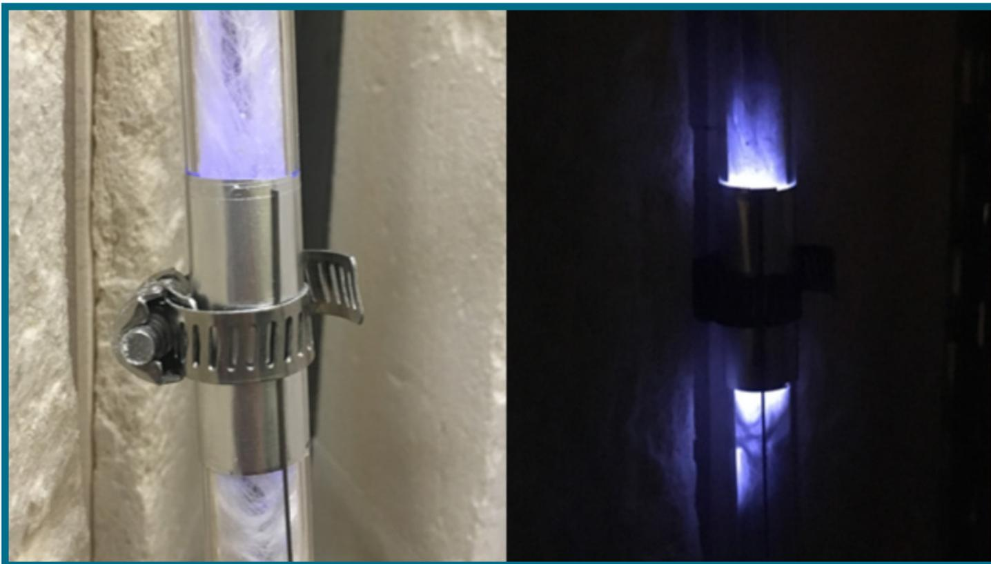
Left - Photo of the produced sulfur. Right - Photo of the plasma discharge.
